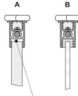
Expansion gap taken into account when calculating the height of chipboard
