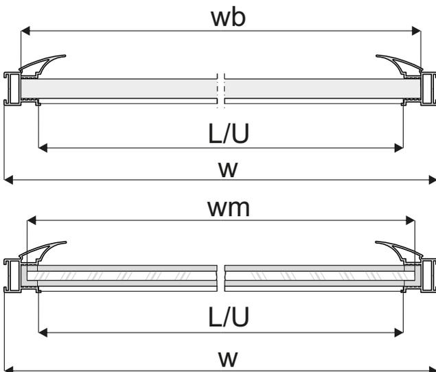
Dimensions helpful during installation of horizontal mid-rails in Simple 10 Frame systems
